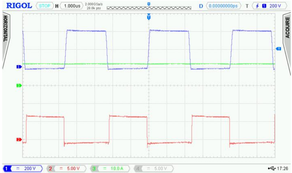
Figure 4-3: Channel 1(Blue): HB switching node (200 V/div); Channel 2(Red): Gate voltage of the Low side GaN device (5 V/div); Channel 3(Green): Load current (10 A/div); time: 1 μs/div.
