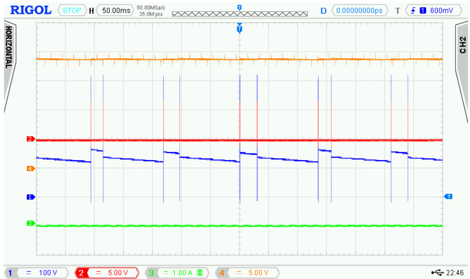
Figure 4-4: Channel 1(Blue): HB switching node (100 V/div); Channel 2(Red): Gate voltage of the Low side GaN device (5 V/div); Channel 3(Green): Load current (1 A/div); Channel 4(Orange): Output Voltage (5 V/div); time: 50 ms/div.
