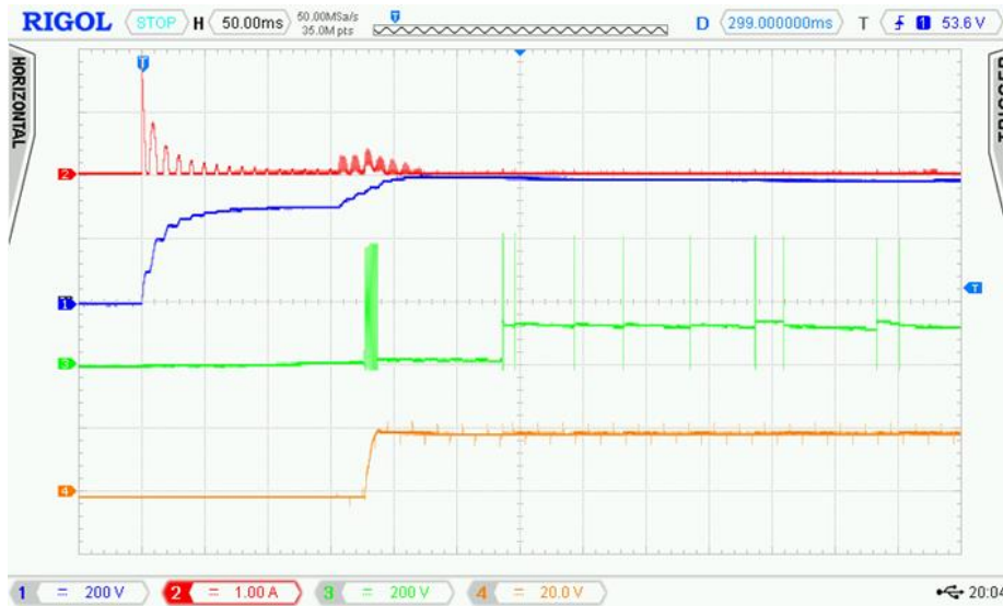
Figure 4-6: Startup waveforms using front end PFC. Channel 1(Blue): Input voltage (200 V/div); Channel 2(Red): Input Current (1 A/div); Channel 3(Green): LLC HB switch node voltage (200 V/div); Channel 4(Orange): Output voltage (20 V/div); time: 50 ms/div.
